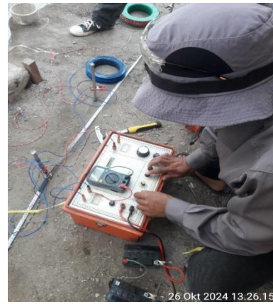
Gambar 5. Pengoperasian Alat Geolistrik/Resistivity Meter Naniura NRD-300 Plus
