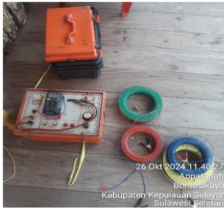
Gambar 3. Alat Geolistrik/Resistivity Meter Naniura NRD-300 Plus
